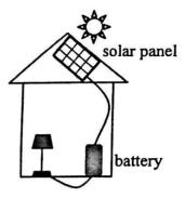
The solar panel of area 1.65 m<sup>2</sup> is connected to the battery via a charger controller (not shown in Figure 3.1). The solar panel delivers 300 W when it is normal to the Sun on a sunny day. Given: solar radiation power per unit area received on the Earth's surface = 1000 W m<sup>-2</sup>
