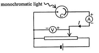
Monochromatic light of fixed intensity is shone on the cathode C of a photocell. The p.d. V applied across the photocell is adjusted and the corresponding current I is measured. What will be the graph of I against V?
