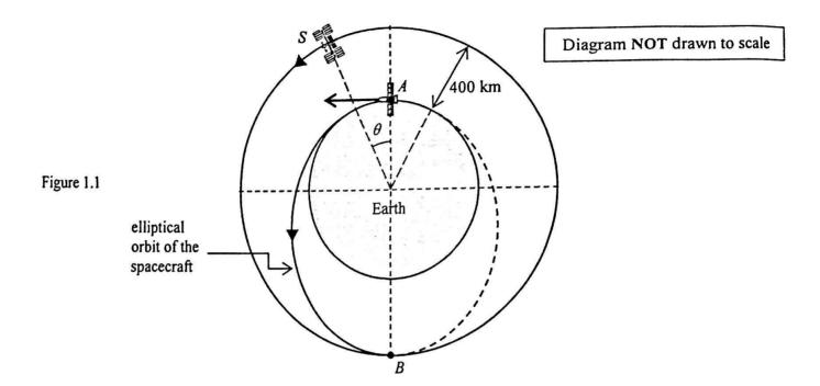
A spacecraft is launched with speed 8.02 km s<sup>-1</sup> from A at the Earth's surface to meet the station S through an elliptical orbit with AB as the major axis. The spacecraft's rocket engine is shut when it coasts from A to B along the elliptical orbit. Assume that the two orbits are in the same plane.
